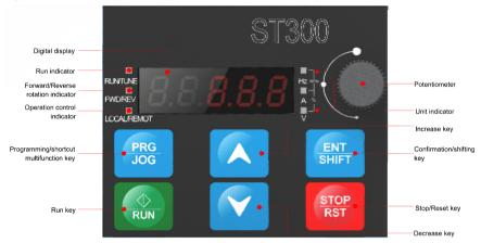
Figure 5-1 Standard LCD keypad
